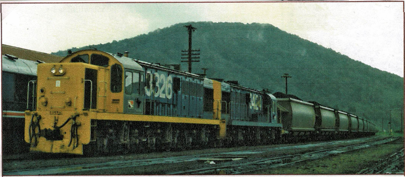
Photo from "The West Coast Coal Route" NZ rail Observer "Leaving Stillwater with an eastbound coal train on 20 October 1988" Wagons are the new aluminium wagons tare 15 tons + 42 tons of coal. Each coal train could transport 1000 tons. At Lyttelton, it was stockpiled and moved by conveyor to the ships
